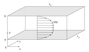
Figure 3: Schematic of channel flow. Fluid flows between two rigid walls at y=a and y=b. The boundary conditions are periodic in x and z and no-slip at the walls. The mean flow U(y) is driven in the x-direction by a mean pressure gradient.
