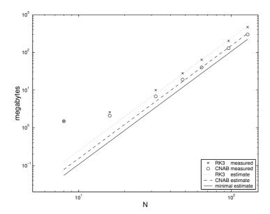
Figure 6: **Memory consumption as function of gridsize.** Comparison of actual memory consumption to scaling-law estimates.
