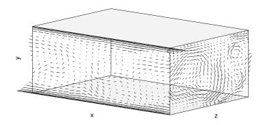
Figure 1: Plane Couette flow simulated with channelflow. The flow is driven by the motion of the upper and lower walls, which travel with equal speeds in the  $\pm x$ -directions. The flow is periodic in x and z. The Reynolds number based on channel half-height and wall velocity is 600. The flow was integrated on a  $24 \times 49 \times 24$  grid with a variable timestep  $0.05 \le dt \le 0.15$ . The plot shows segments of streamlines confined to the exposed planes.
