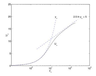
Figure 5: The law of the wall. Mean velocity of a turbulent channelflow compared to scaling laws for the viscous sublayer  $(U/u^* \approx y_+)$  and the inertial layer  $(U/u^* \approx 2.5 \ln y_+ + 5)$ .
