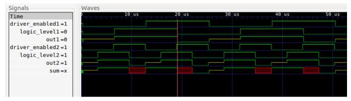
driver\_enabledX (X is 1 or 2 for core 1 or core 2) shows the pin from the port driven by coreX - this represents DDR bit. logic\_levelX represents the setting of PORT bit. outX represents the resulting signal from above values.
