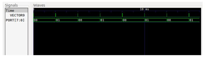
Let's look on a detail. You can see, how long the interrupt procedure was running and when the port value was changed. Compare it with the print out on standard out before! (in picture the value for "Marker:")
